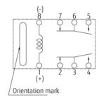
PC board mounting pad layout (TOP VIEW)
