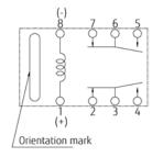
PC board mounting pad layout (TOP VIEW)
