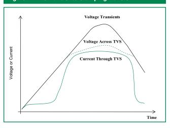
Figure 2 - Peak Pulse Power Rating
