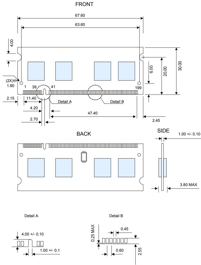
Note: All dimensions are typical with tolerances of +/- 0.15 unless otherwise stated.
